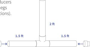
5. Fuse the two 3-inch to 3-inch connectors together.
