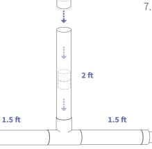
7. Place the end cap on the top of the station. Attach a service container label near the top of the bait station.
