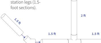
5. Place the two remaining 1.5-foot sections on the ends of the 45° connectors.
